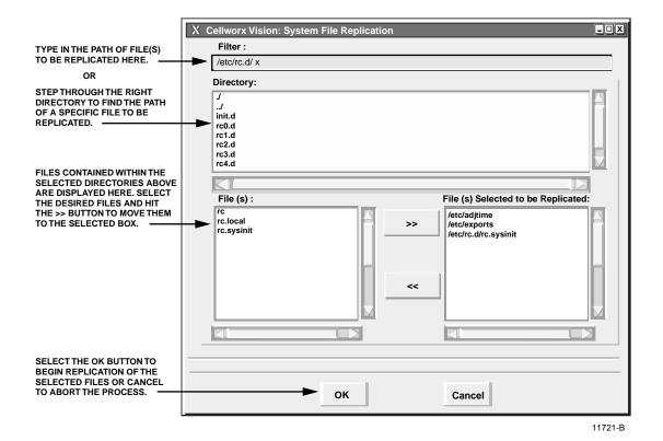
Figure 722-2. Cellworx Vision system File Replication Window
